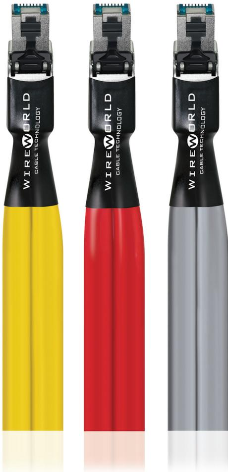
**W**ireworld Ethernet cables use an innovative flat design to support next generation Category 8 transmission speeds while providing greater flexibility and ease of use than conventional round Ethernet cables. Even though they have full sized 23 gauge conductors and triple-shields on each conductor pair, this patent pending Tite-Shield design is just a tenth of an inch thick. This elegant cable structure also simplifies assembly with Wireworld shielded RJ-45 plugs.
